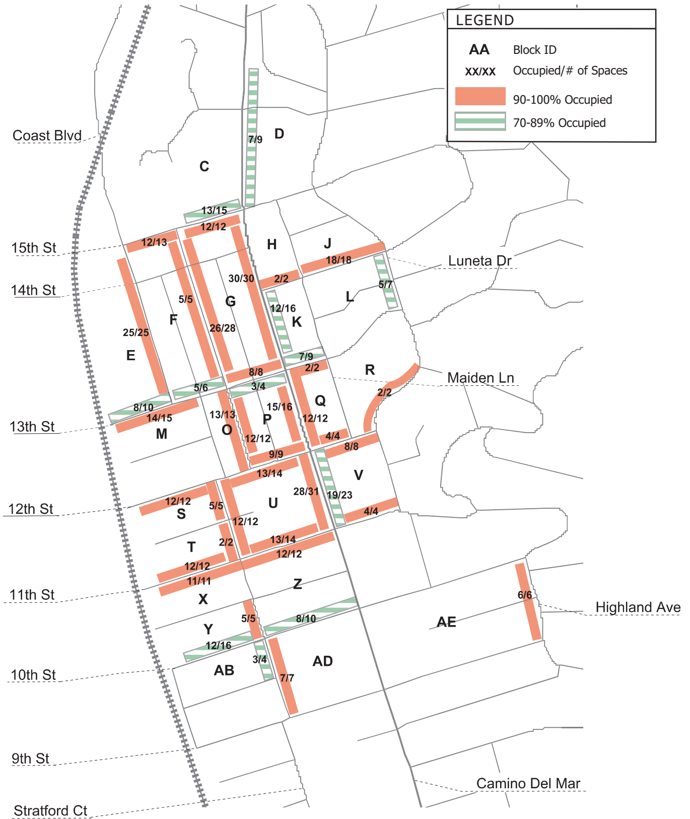
Figure 4 Weekend Peak Hour (1 PM) On-Street Parking Occupancy
