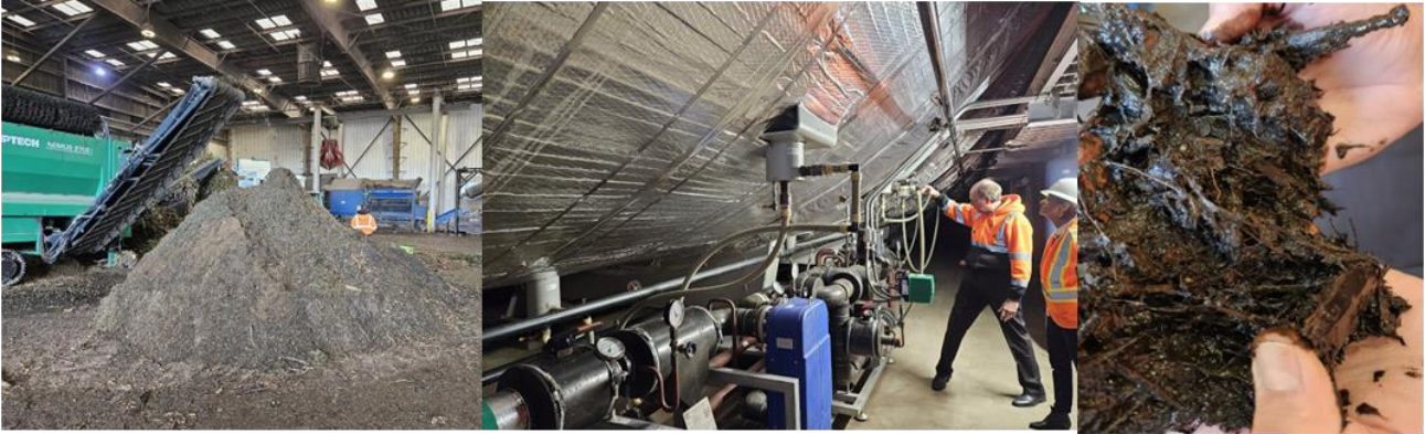
On the left, commingled green yard cuttings and solid kitchen waste mechanically shredded after arrival at the facility. In the center, under the belly of one of the anaerobic digester. On the right, "digestate" as it exits the digester. It is used as fertilizer by local farms.
