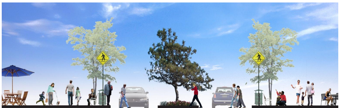
VSP Figure IV-5, Crossing distance reduces from 80 feet to 34 feet: New plazas are provided at corners.
