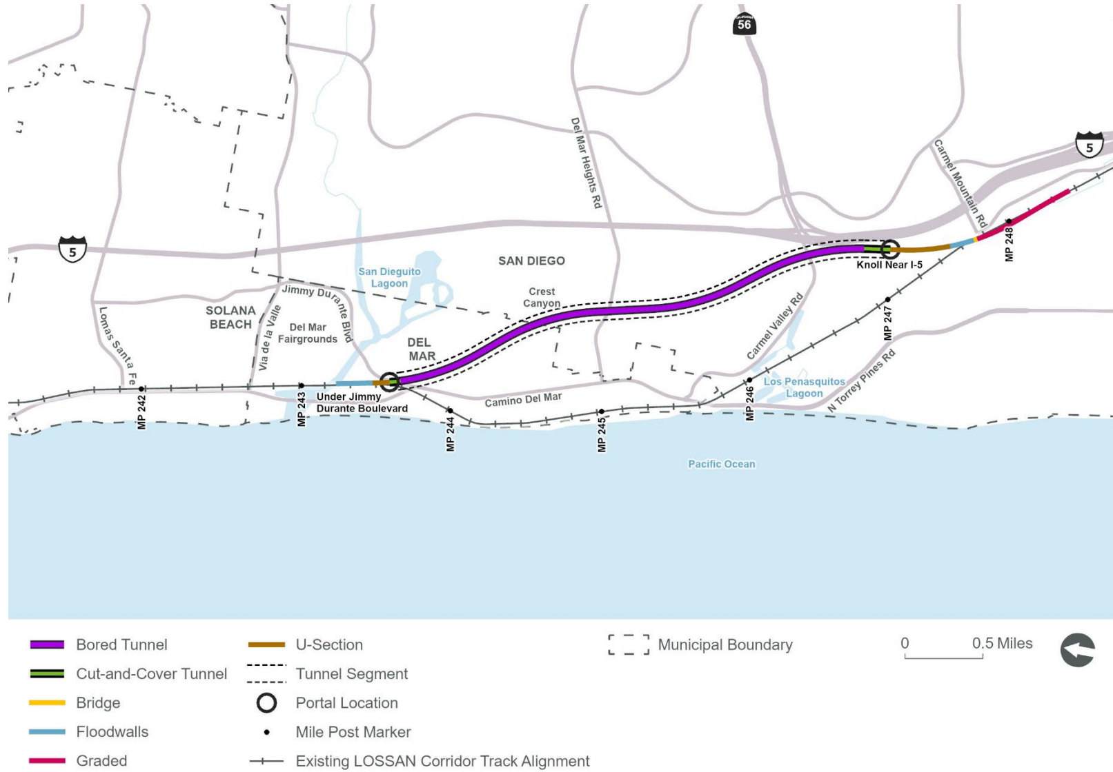
Figure 5. Under Crest Canyon Alternative Alignment
