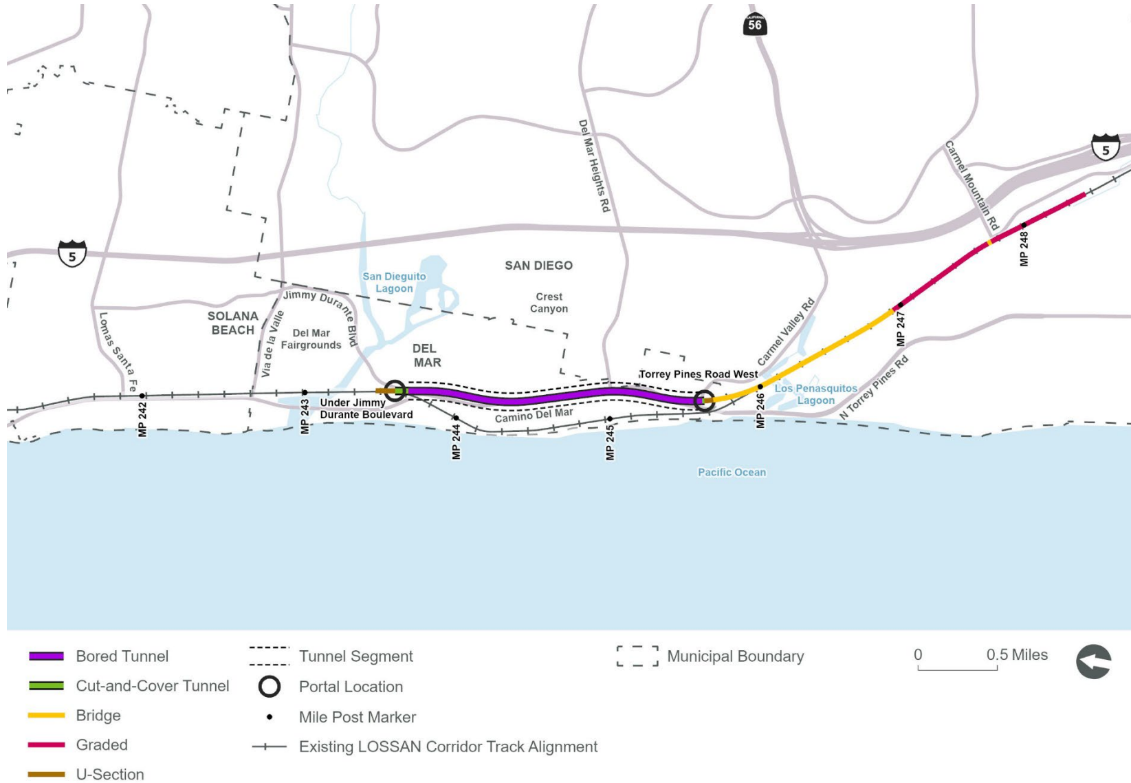
Figure 6. Under Camino Del Mar Alternative Alignment
