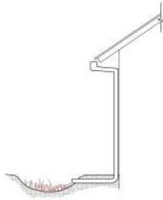
Connecting a roof leader to a self-retaining area. The head from the eave height makes it possible to route roof drainage some distance away from the building.
