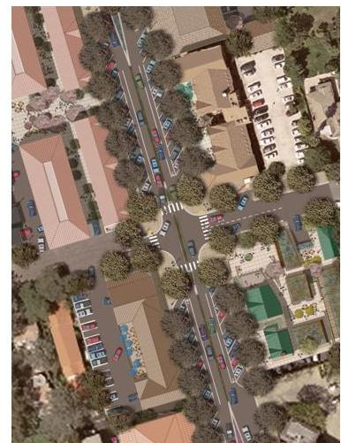
Streetscape improvements to Camino del Mar allows for an increase in on-street parking with 30 new parking stalls. A public parking structure will provide additional off-street parking.
